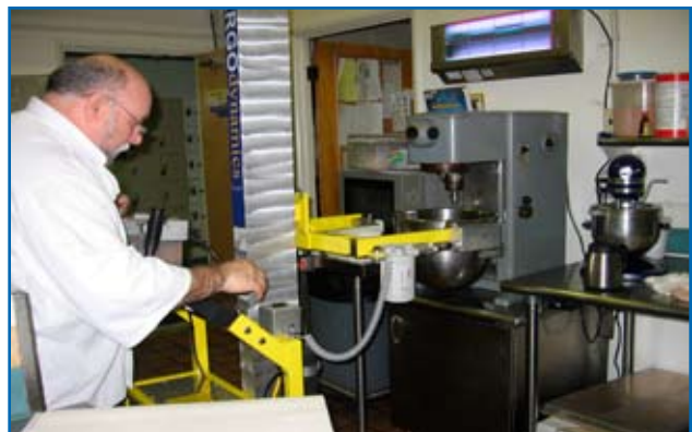
Go-lift removing full mixing bowl from machine
